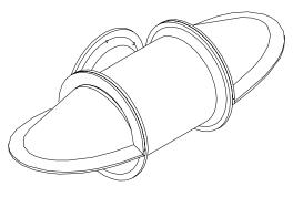
A standard Sidepower sternthruster tunnel with the add-on cowls for shallow installation.
